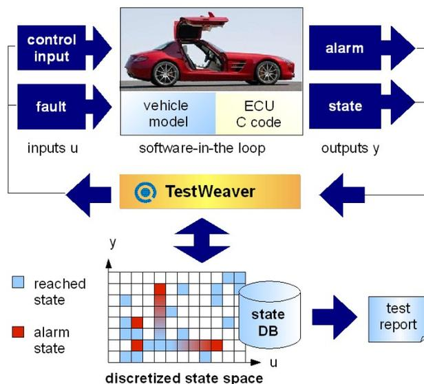
Fig. 6: Setup of the automated DCT software test
