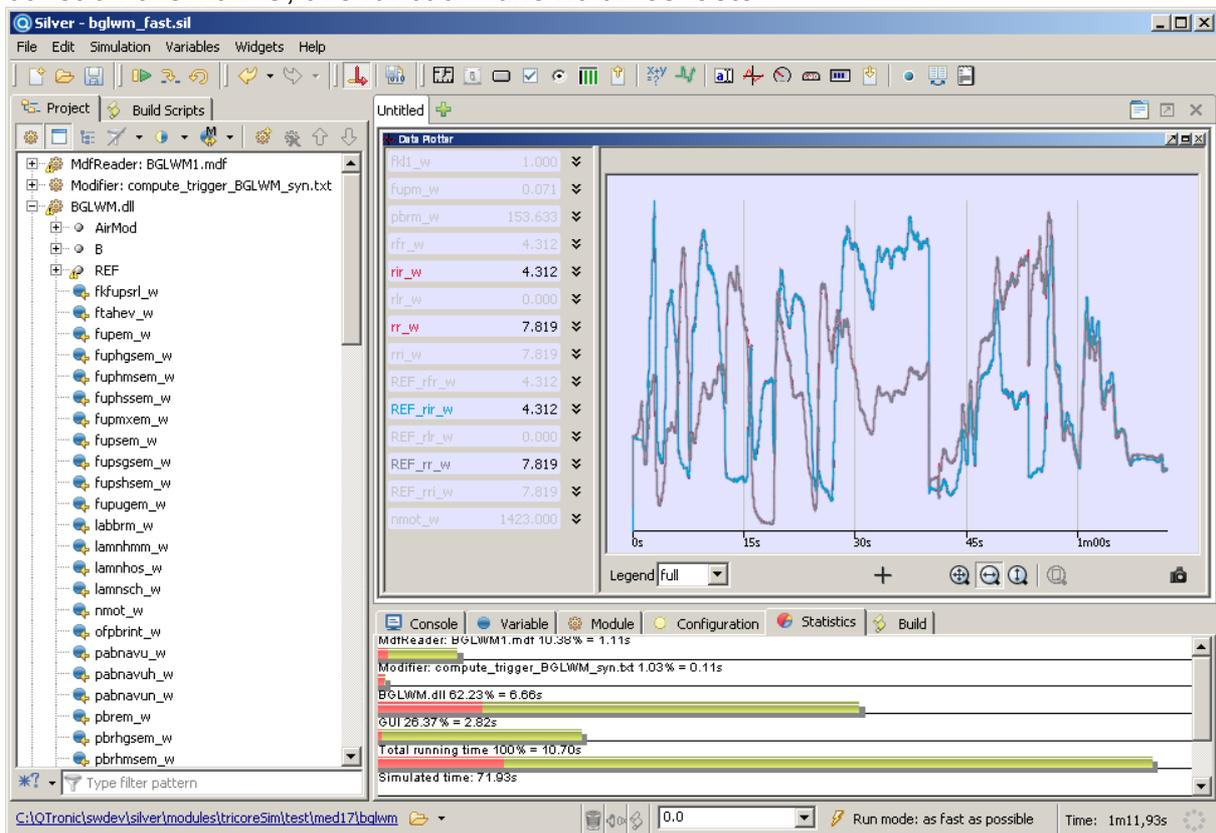
Fig 2: The BGLWM function running in Silver, driven by measurement file
